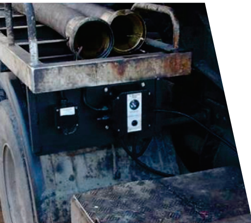
Earth-Rite II MGV 静电接地系统可以安装在吸污槽车和槽车上
