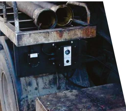
Earth-Rite II MGV 静电接地系统可以安装在吸污槽车和槽车上
